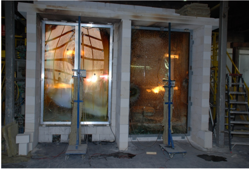
Figure 4: Test specimen in front of furnace in modified setup
