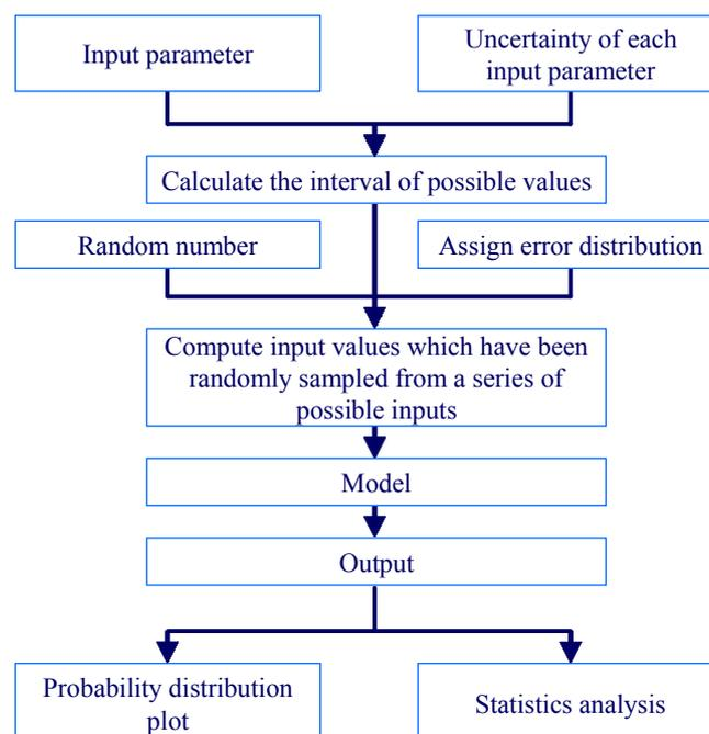
Figure 6: Process flow of the Monte Carlo tools
