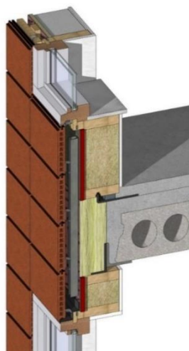
Figure 1. Combustible materials protected by EI15-rated cladding (see cladding marked in red).
