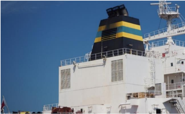
figure 1: funnel and machine house ventilation grids
