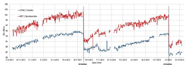
Figure 2. An example of the increase of noise level due to rail roughness and the effects of grinding for two types of light rail vehicles.
